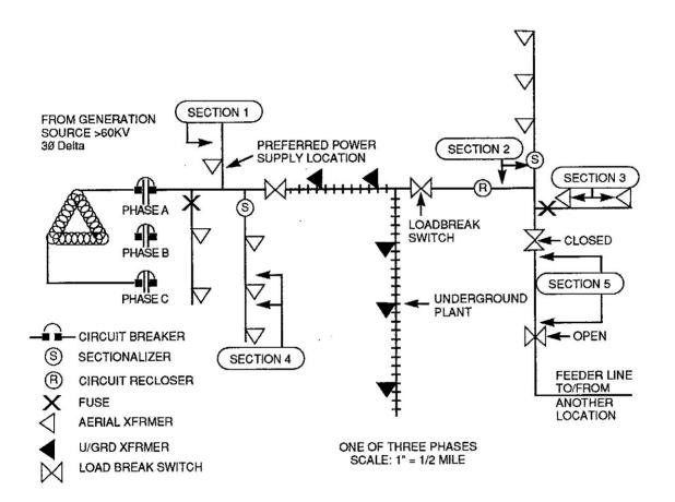
Figure 1 - Typical Power Distribution System
