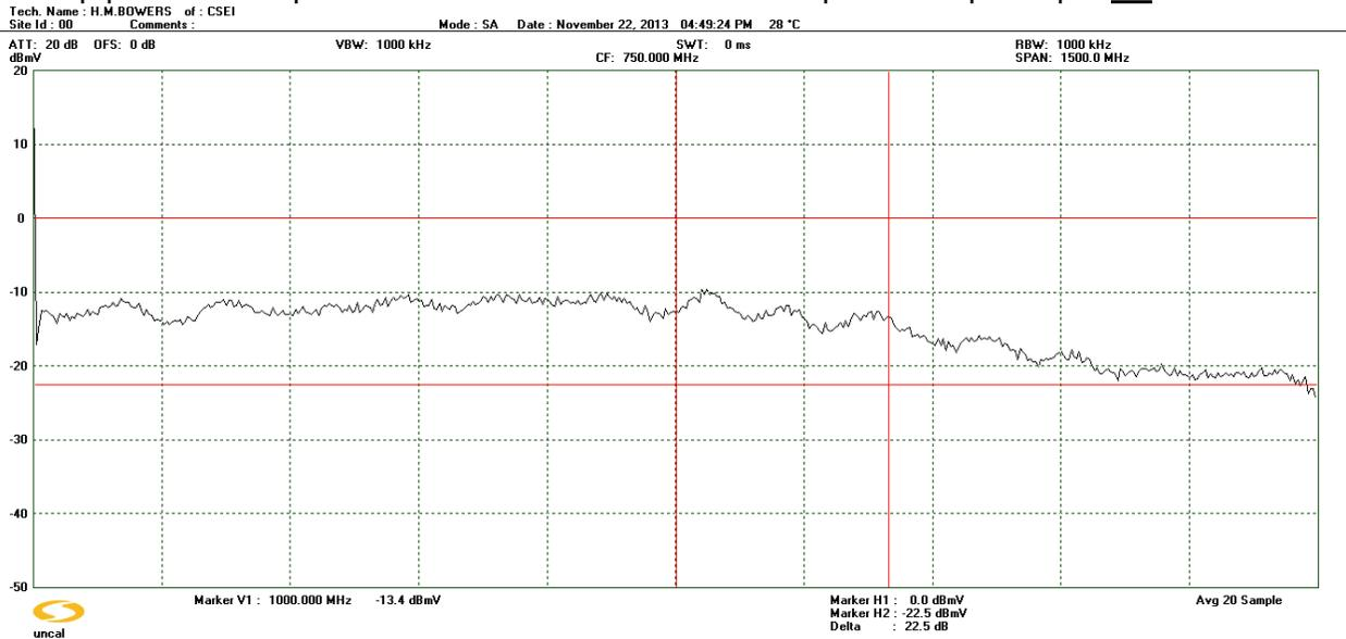
Isolation between the tap port and thru port with the input un-terminated is poor, but considered an improvement over the 2-way splitter under similar poor impedance match conditions. This illustrates why directional couplers offer improved isolation performance as compared to splitters when used in 'combining networks'.
