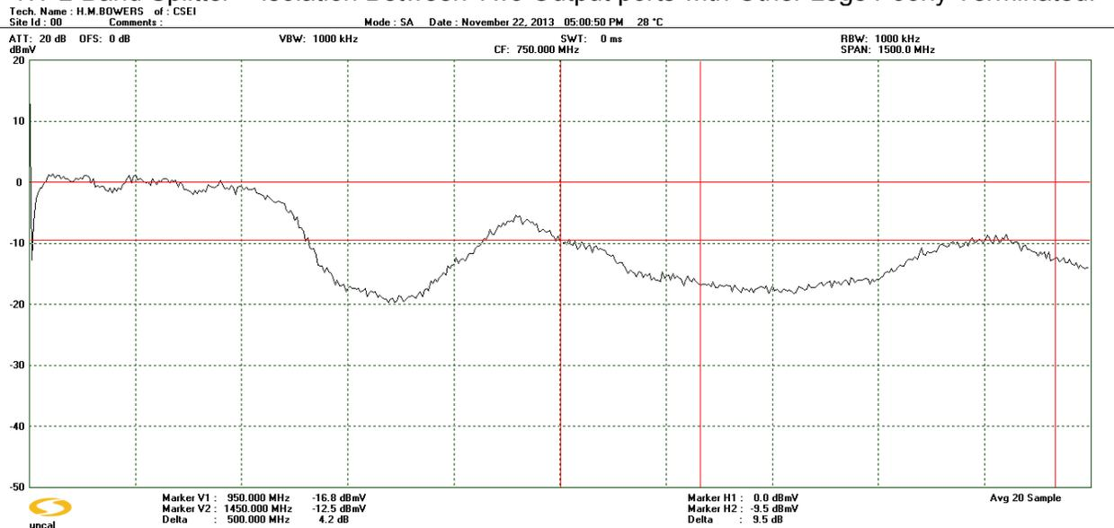
Port-to-port isolation varies from approx. 10 dB to 17 dB in the band of interest; however it can be seen that isolation at other frequencies is very poor, with the isolation at essentially zero dB from 0 to 300 MHz!
