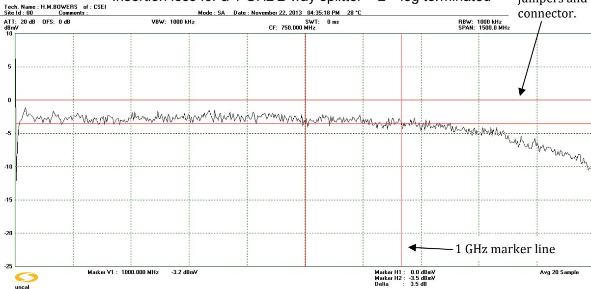
The red line at 0 dBmV marks the baseline (jumper from noise generator to analyzer input using short cables and a F81 connector) response of the noise generator out to 1.5 GHz and beyond. The black line represents the throughput loss from splitter input through one of the two output legs, with the other output properly terminated. Loss at 1 GHz is approx. 3.5 dB! The loss at 1.5 GHz, however, is >10 dB!
