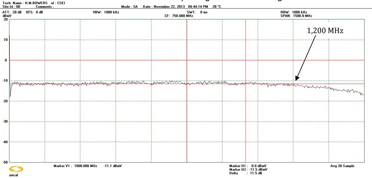
The insertion loss at 1 GHz is 11.5 dB on the tap leg. The tap leg response is flat to 1.2 GHz!
