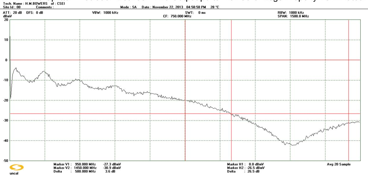
Between 950 to 1450 MHz, port to port isolation varies from 27 dB (950 MHz) to approx. 42 dB (approx. 1,200 MHz) depending on the frequency of measurement.
