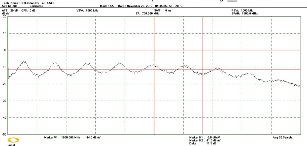
Again, large response variations and a distinct standing wave pattern are seen in the tap leg feed when the thru-leg has a poor impedance match.
