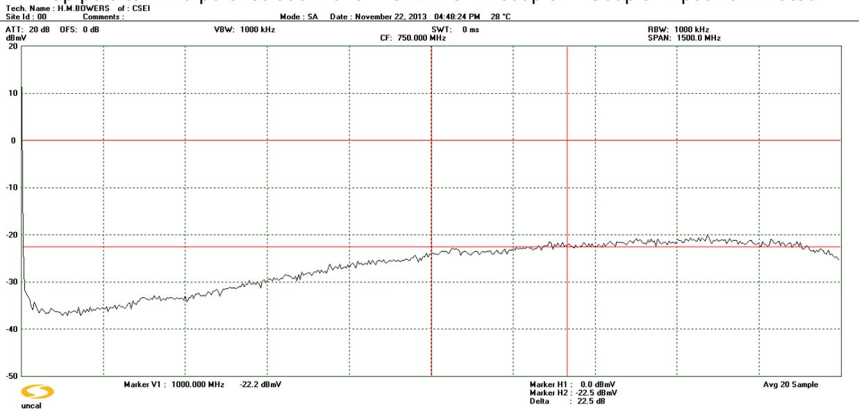
Tap to output port isolation varies from approx. 23 dB (at 1 GHz) to 36 dB (at 75 MHz) depending on the frequency measured. This is similar to, but considered an improvement over, the isolation measured on the 2-way splitter.
