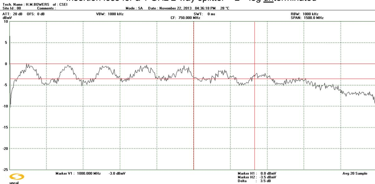
This response trace shows loss through one of the 2-way splitter legs, with the other side unterminated. Note the distinct standing waves in the throughput response. Also note that at some frequencies the 'thru loss' is almost 0 dB, while at others it is at 6 dB, due to signal reflections from the unterminated leg and poor isolation between ports.
