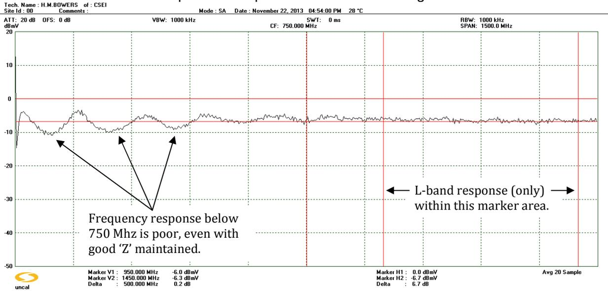
Actual 950 to 1450 MHz response is between two red vertical markers, with insertion loss at 6.7 dB.
