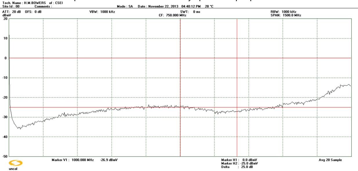
The worst-case (poorest) port-to-port isolation below 1 GHz occurs from approx. 600 to 750 MHz and is 25 dB. The splitter input is properly terminated.
