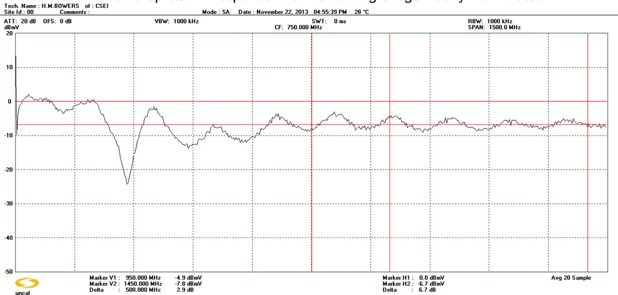
The L-band splitter is not as badly affected by poor termination on the remaining legs *in the 950 to 1450 MHz range*; however peak/valley response variation is still 3 to 5 dB.
