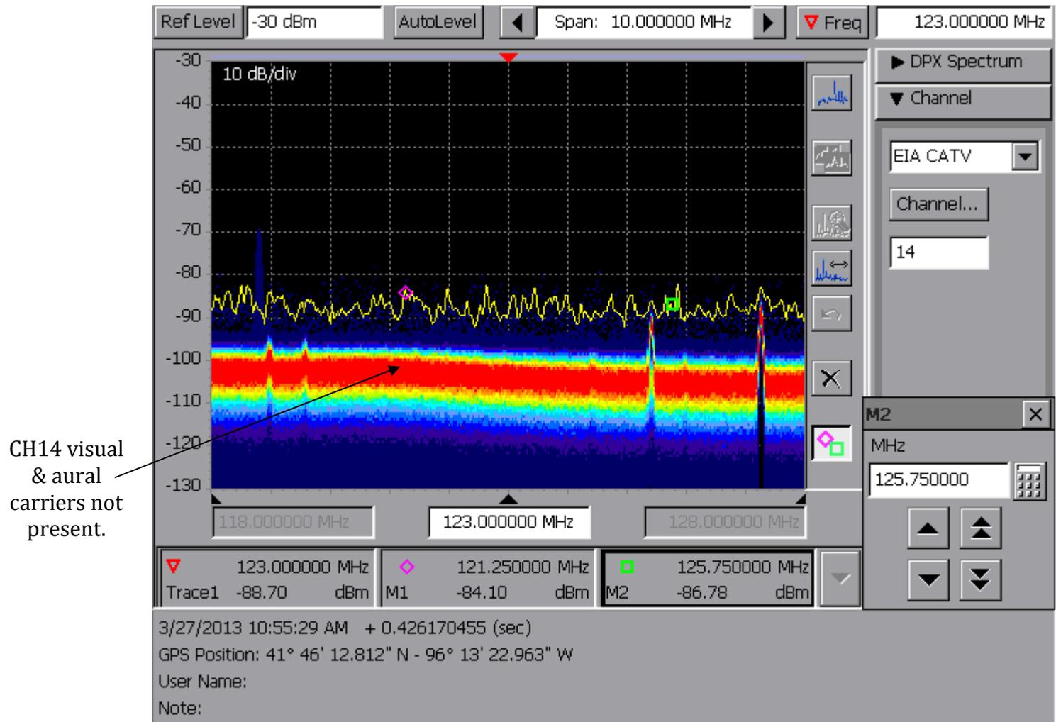
**Test Location #2:** Measuring at the same physical location but in the CH14 spectrum, even though the leakage levels were greater at CH117 at Test Location #1, no leakage is evident. This was the 'norm' (except for several locations); many low-level leaks were measured at CH117 but it was rare to see *any correlating leakage* in the 108 to 137 MHz aeronautical region.
