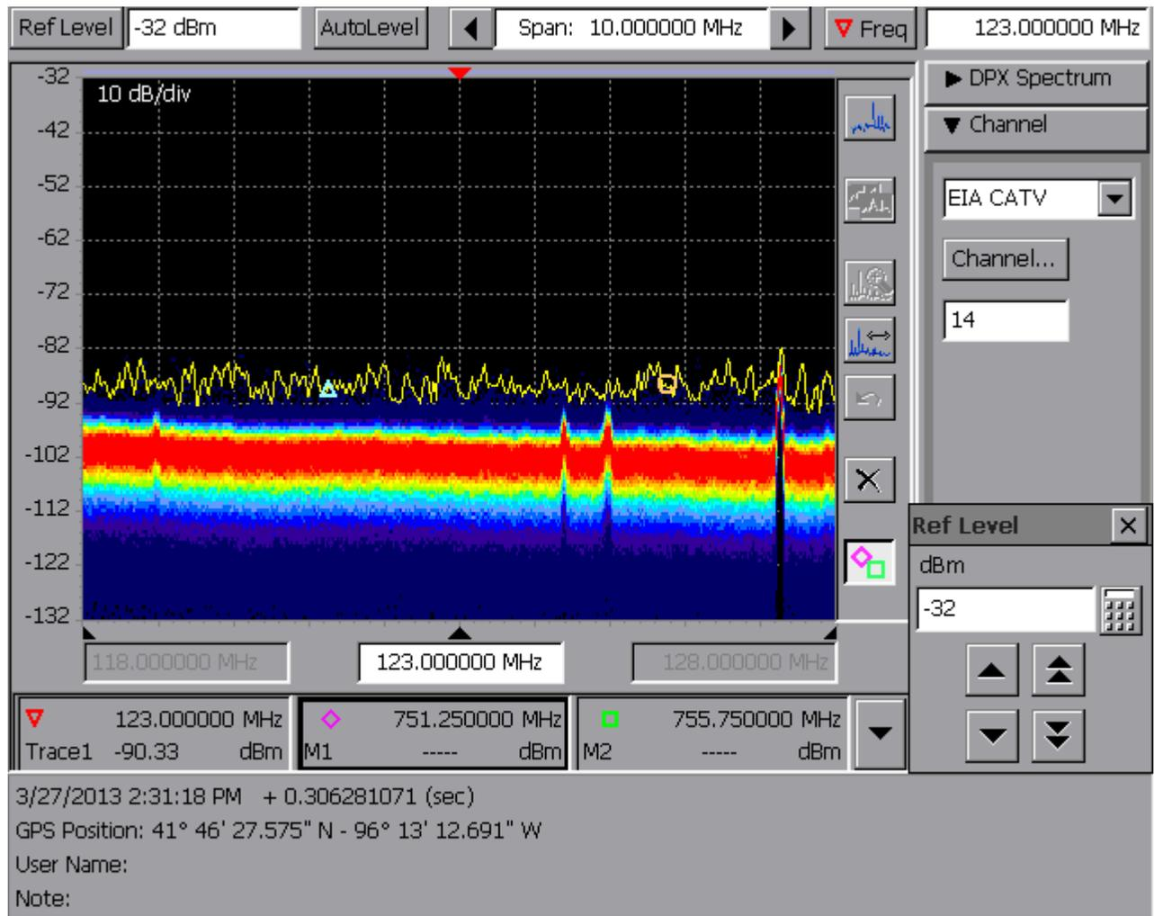
**Test Location #4:** This screen capture at the same location shows no leakage at CH14, although there were times when I saw the CH14 luminance carrier briefly 'come and go' (at blue triangle marker).
