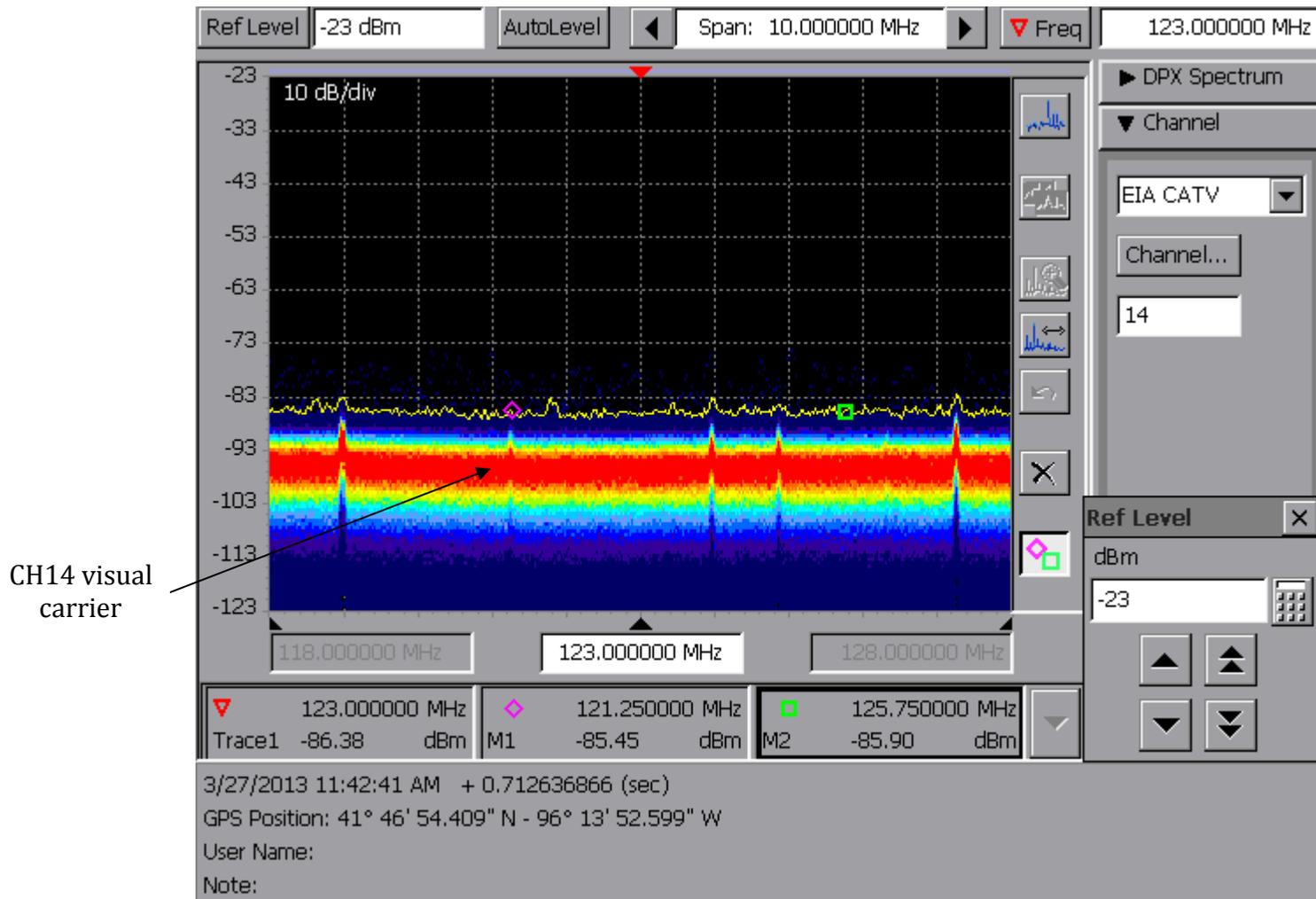
**Test Location #1:** This DPX screen shot is at the same CH117 low-level leak location; however now I'm measuring CH14. This location was a bit unusual, in that the CH14 visual carrier (purple diamond marker) is just barely visible, just 'poking' out of the thermal noise floor. Most leaks of this amplitude at CH117 (there were many) showed no corresponding leakage at CH14.
