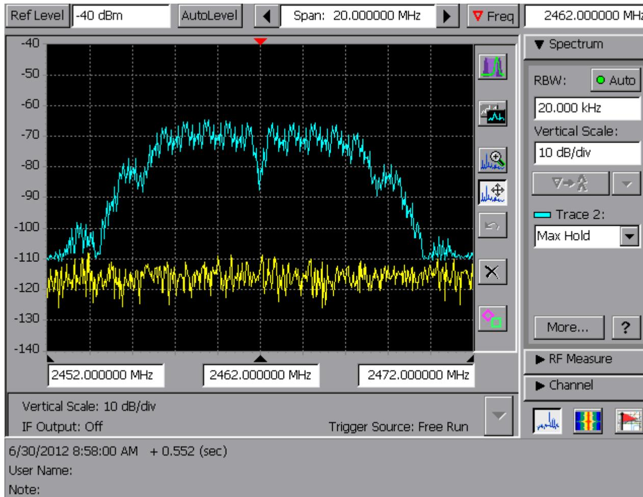
I've reverted back to standard frequency analysis mode, with a 'real time and peak hold trace', to demonstrate that without the spectrogram or DPX views, it's very difficult to determine any sort of problem within the WIFI spectrum. The beat is too low to see with the real time trace, and peak-hold obviously will not show a beat unless it's amplitude exceeds the amplitude of the desired signal. Basically, everything looks fine here.
