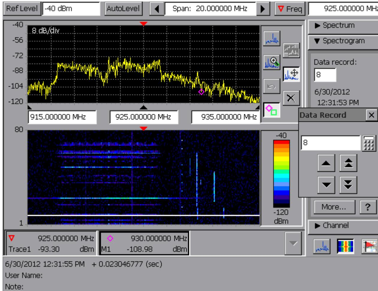
In the 1st Quarter 2012 Technical Report we examined some very active spectrum from 915 to 935 MHz. Selecting data record 8 in the spectrogram above, we can see considerable spectral activity. The spectrum from approx. 917 to 927 MHz 'appears' to be digital in nature (QAM, VSB, PSK, etc.), along with what appears to be many low level analog carriers in the 929 to 934 MHz region.
