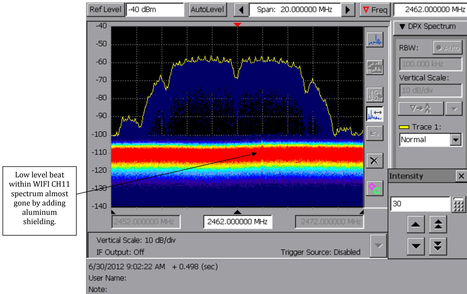
Note that the beat is now significantly reduced in amplitude through the addition of some aluminum shielding between the antenna and interfering source direction.
