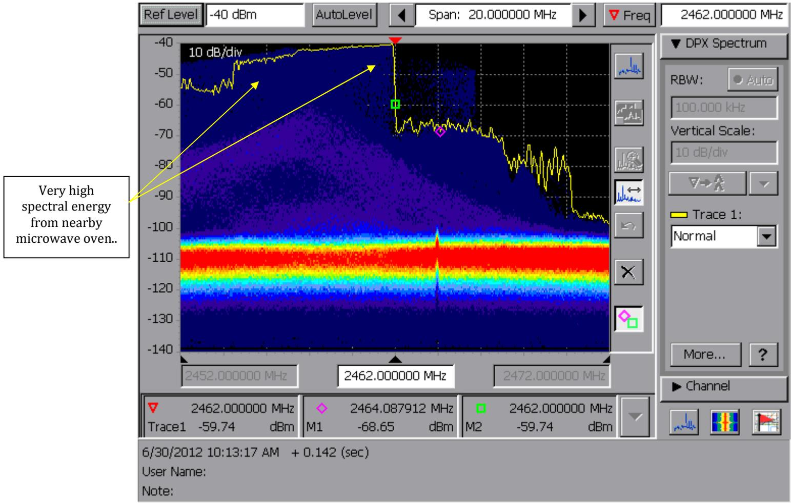
Finally, the above shows the spectrum around WIFI CH11 with a microwave oven running approximately 20 ft away. Note that the lower spectral portion of CH11 is completely overridden by energy from the nearby magnetron. Compare this with previous DPX waveforms for WIFI CH11.
