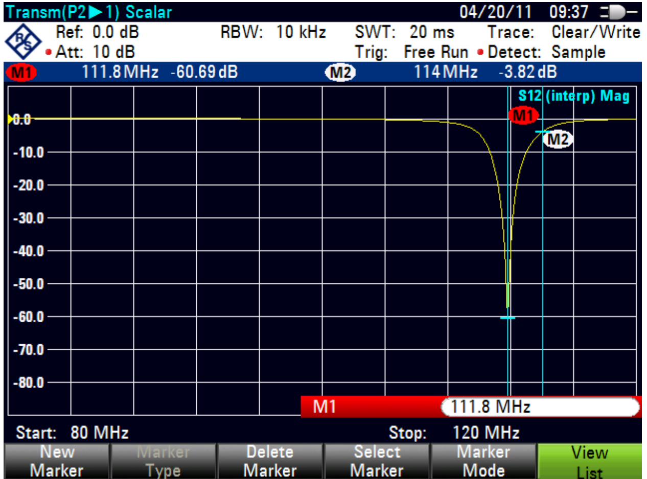
Response (scalar) of a CH98 sample trap. Notch depth at the interfering carrier is -60.7 dBc, and insertion loss at the adjacent carrier band edge is 3.8 dB (much greater than others)!
