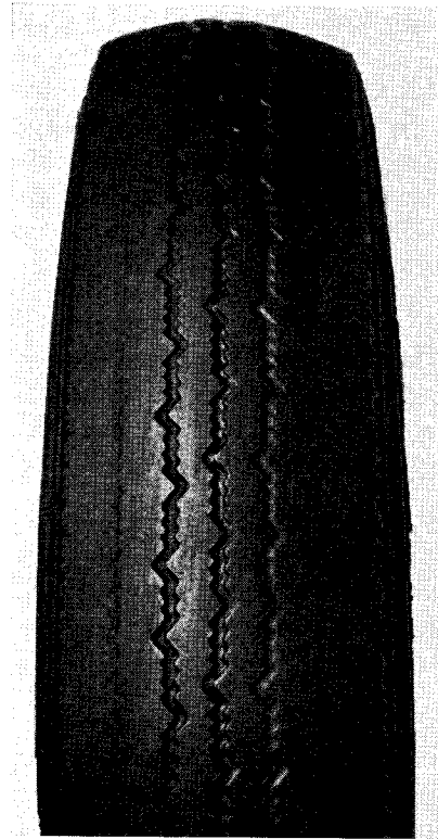
Fig. 2. Excessive tyre distortion from persistent underinflation causes rapid wear on the shoulders and leaves the centre standing proud.
