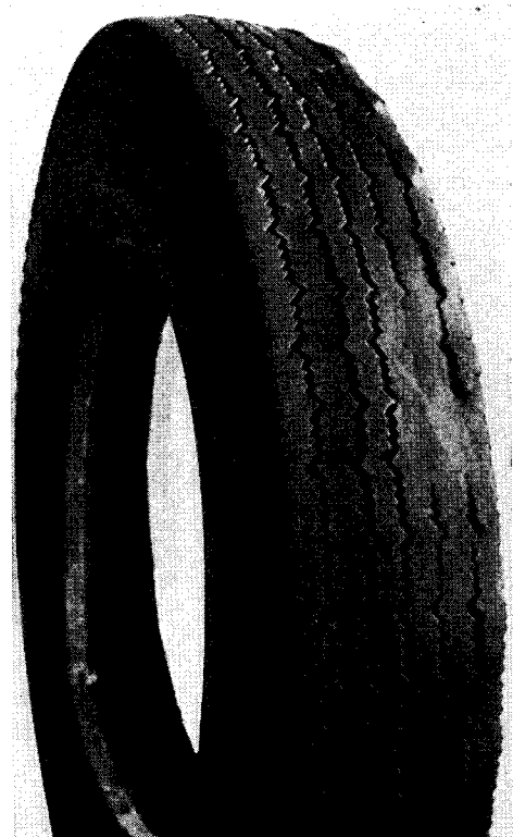
Fig. 8. Irregular “ spotty ” wear, to which a variety of causes may contribute.
