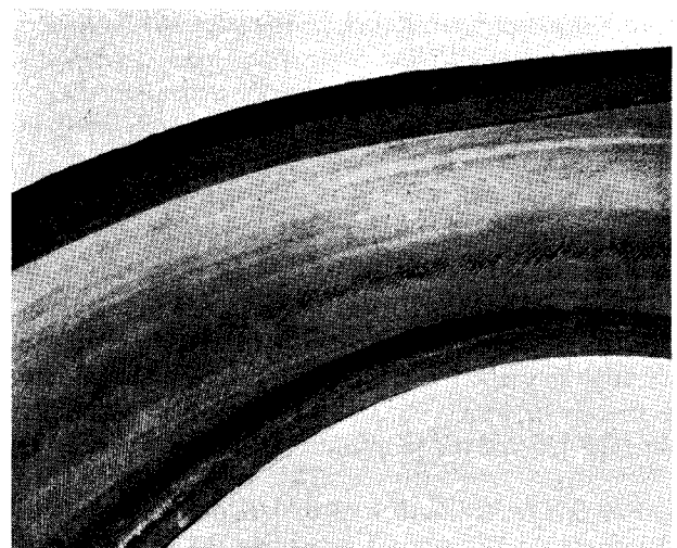
Fig. 3 The case is breaking up due to over-flexing and heat generation.
