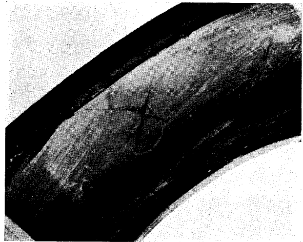
Fig. 6. Severe impact has fractured the casing.
