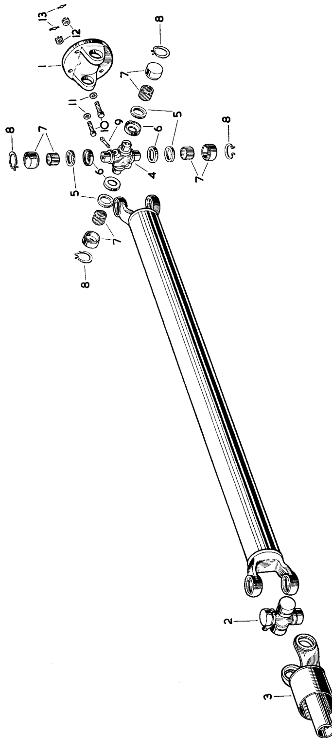
Fig. 2. Exploded view of propeller shaft assembly (Standard trans- mission propeller shaft illustrated).
