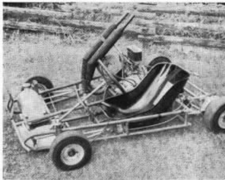
Culverite Sidewinder with 41 Rhp at 9000 rpm 297 cc Yamaha twin
