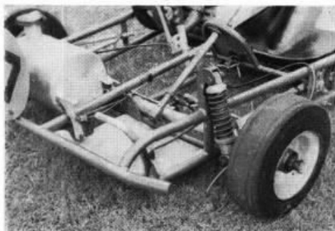
Front suspension on the Culverite Sidewinders. The clutch lever is on the gear lever
