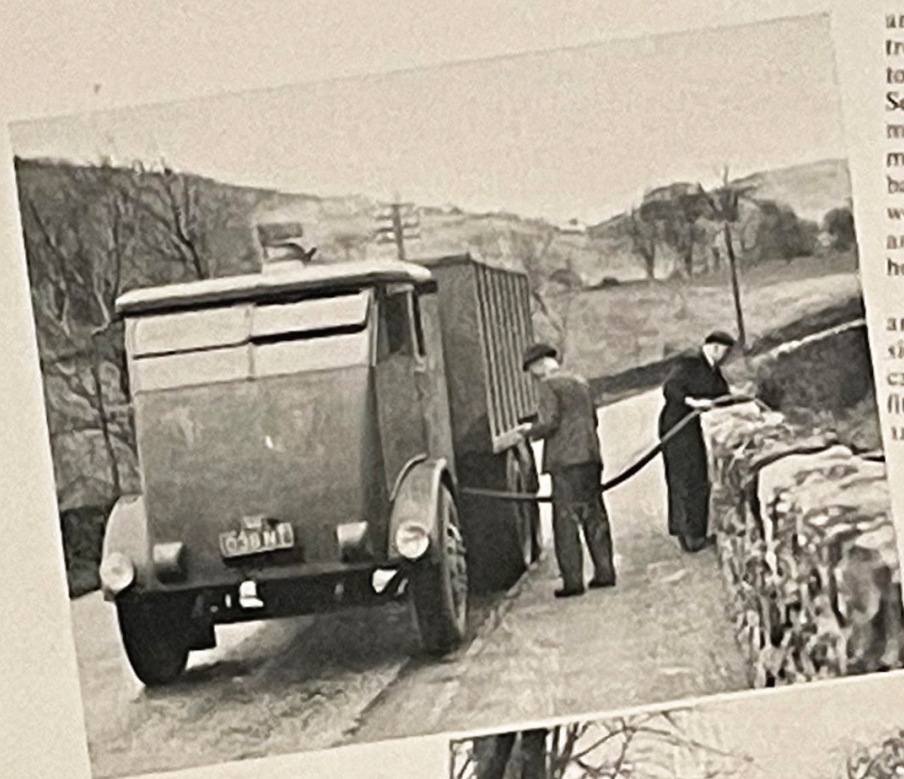
After turning in Llangollen, a stop was made at a stream for replenishment of water supplies. The reserve supply was not used in 32½ miles of normal operation.
