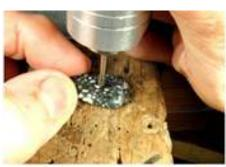
One of the things my students often ask to do is drill a hole through a piece of gemstone. The usual thought is to get a diamond drill, but I've been disappointed with them. I think the reason is that the tip of the drill is just pivoting in the hole and fails to cut well. When it looks like the drill isn't cutting, the tendency is to push with more force. The drill gets hot, and the diamond grit falls off.
