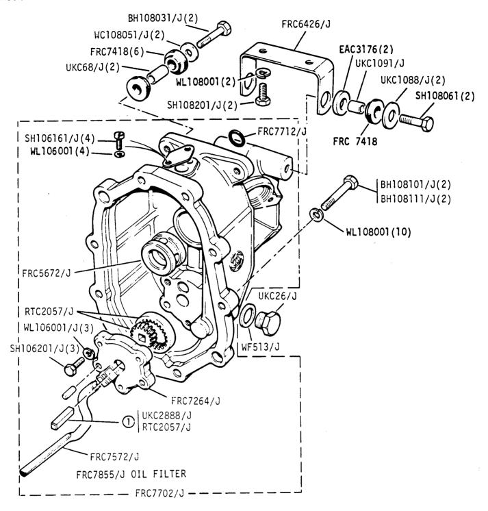
① RTC2057 - Gear Kit Oil Pump
