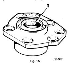
Clamp caliper mounting bracket between protected laws of vice.
