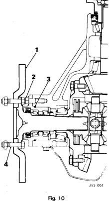
Cut locking wire and remove five set bolts (2, Fig. 10) securing caliper mounting flange to final drive. Withdraw complete output shaft assembly and discard 'O' ring (3, Fig. 10).
