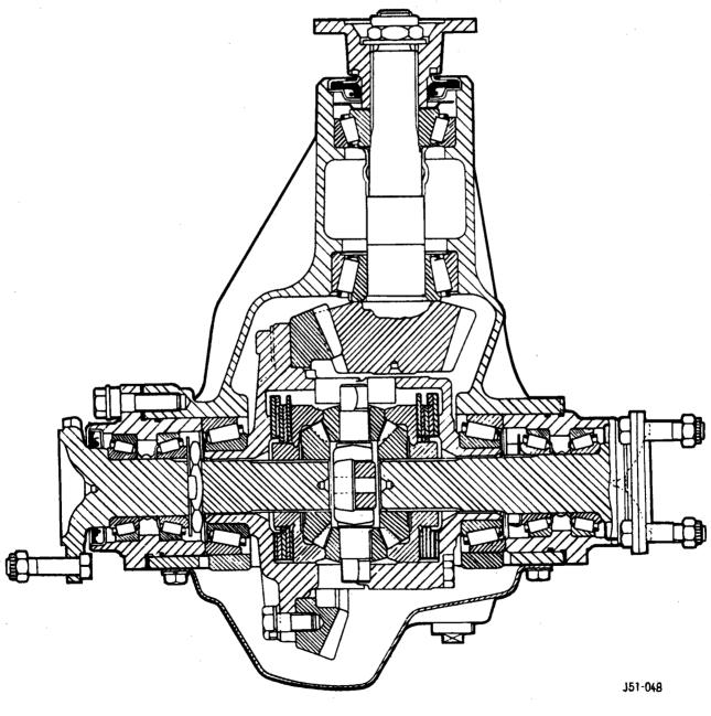
CROSS-SECTION OF THE LIMITED SLIP REAR AXLE
