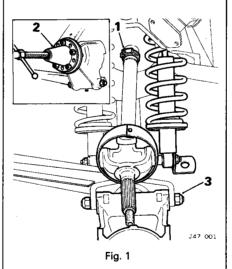
Remove grease nipple from hub carrier, and using tool JD 1D (2, Fig. 1), withdraw hub from shaft. Allow the hub carrier to pivot about wishbone pin. Before detaching inner joint, release lower end of rear spring/damper unit (3, Fig. 1) and swing aside to clear joint. Collect and retain any camber setting shims fitted between inner joint and brake disc.
