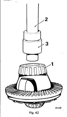
Place the differential assembly with the bearings in their housing into the differential case without the pinion in position.
