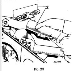
inner universal joint shrouds and slide the shrouds outwards.
