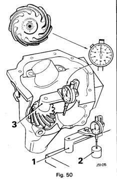
Adjust bracket carrying dial indicator using 4HA setting block. For differentials with a white painted circle on the rear cover use tool no. SL3-2. (2, Fig. 50) and set dial face to zero.
