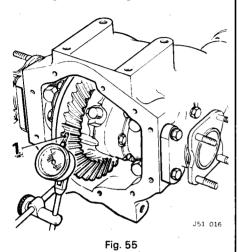
Move drive gear by hand to check backlash which should be 0,15 to 0,25 mm (0.006 to 0.010 in). If backlash is not to specification, transfer the necessary shims from one side of the differential case to the other to obtain the desired setting. Check backlash in at least four positions of drive gear, ensuring that backlash is always greater than 0,15 mm (0.006 in).
