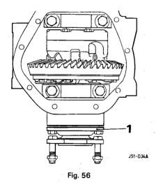
Check that the torque to turn the input flange is 1.4 to 2.8 kgf/m (10 to 20 lbf/in) additional to the torque measured previously to turn the pinion (page 51-15)
