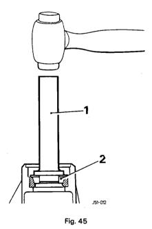
Remove differential assembly from the gear carrier.
