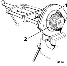
Remove the differential side bearings using tool Nos. 47 (1, Fig. 34), SL 14-3/2 (2, Fig. 34) and SL 14-3/1 (3, Fig. 34), and collect the shims.
