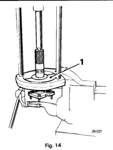
Prise oil seal from caliper mounting bracket. Collect outer bearing and cone. Discard oil seal.
