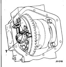
Turn pinion by hand and check run out on back face of gear. Run out should not exceed 0,13 mm (0.005 in). If run out excessive, strip the assembly and rectify by cleaning the surfaces locating the drive gear. Any burrs on these surfaces must be removed.
