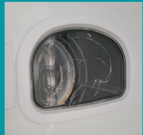
Fourth Floor Diamond Head Dryer - Glass window cracked - discovered Saturday 4/16
