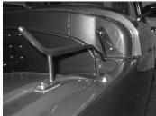
Install roller mount to hood using factory hood bolts. Install mount in center of adjustment, side to side and front to back. Lightly snug bolts.
