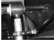
Let the hood roll down slowly. If it doesn't go all the way down, the hood roller mount will need adjusting to let it go down. This can be adjusted to bring the back of the hood up to match the cowl, adjusted sideways to make the side of the hood line up with the cowl.
