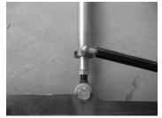
Parallel the tubes to approximately 63 ½" apart center of rod end to center of rod end. Snug the bolts on the hinge bracket.
