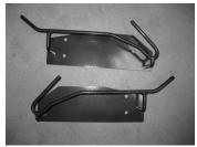
Remove the battery side mount that goes to the inner fender apron if it is still on the truck. Remove the cage nut that is in the inner fender on the passenger side.
