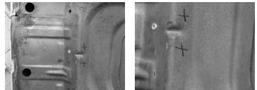
Be careful not to bind the hole saw and dimple the outside of the hood. Install the 3<sup>rd</sup> bolt(5/16") with a flat washer on the bolt along with a flat washer and nylock nut inside of the hood. Install supplied plastic plug after all bolts are tightened for the final time. Repeat for the opposite side.
