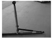
This is important because the gas shocks will push on the jam nuts. If they are installed improperly, they will push on the tubes, loosen the jam nuts and pop the gas shocks out of the mounting balls.
