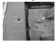
If you want the side battery mount reinstalled, you will need to reshape it and mount it to the side of the new bracket.
