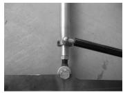
Parallel the tubes to approximately 61  $\frac{1}{2}$ " apart center of rod end to center of rod end. Snug the bolts on the hinge bracket.
