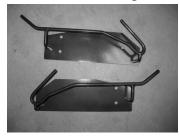
Remove the battery side mount that goes to the inner fender apron if it is still on the truck. Remove the cage nut that is in the inner fender on the passenger side. (This is not on all models)
